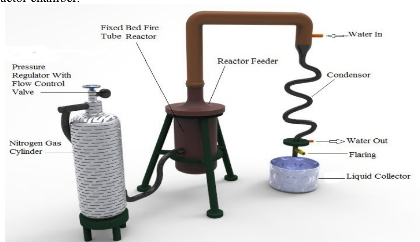
Figure 1: Schematic representation of experimental set-up of the reactor
