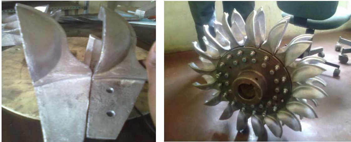
Figure 4: Alignment of buckets on the runner and a complete turbine
