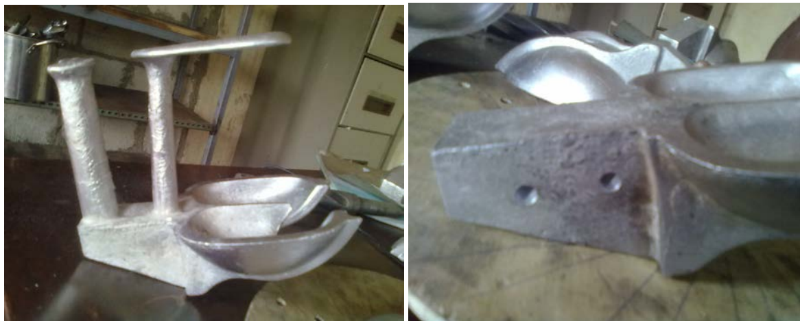
Figure 3: Pelton bucket that has been sand cast and after it has been machined
