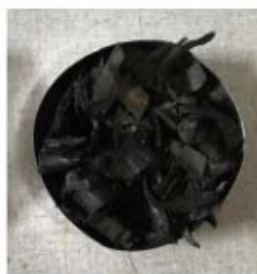
Heated to 500 degrees Celsius in a tube filled with nitrogen
