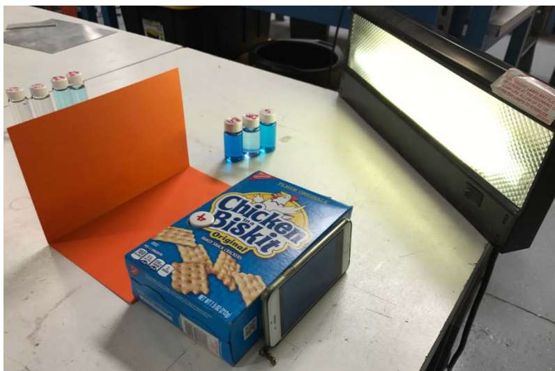
Figure 1. Photo of the absorption measurement setup
