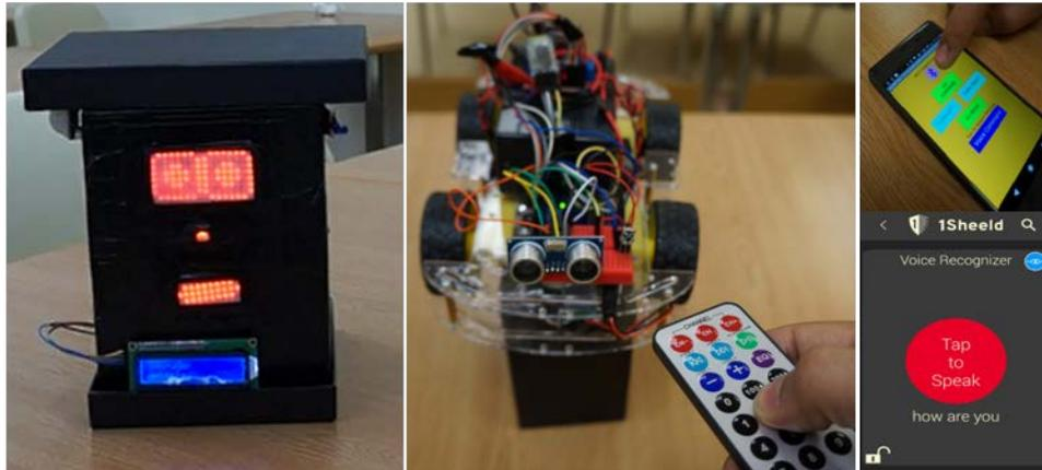
Figure 2. TKFR2: A Multifunction Robot (Face part, Robot part, IR/Mobile App/Voice Command Controls)
