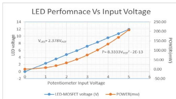
Figure 3: Load performance as a function of Arduino voltage
