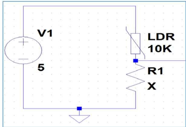
Figure 1: LDR voltage divider
