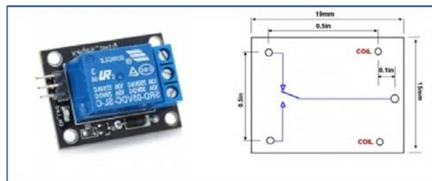
Figure 2: Relay and a circuit diagram [1]
