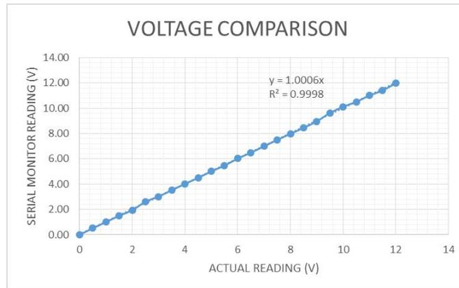
Figure 4: Voltage comparison between Serial Monitor and Battery.
