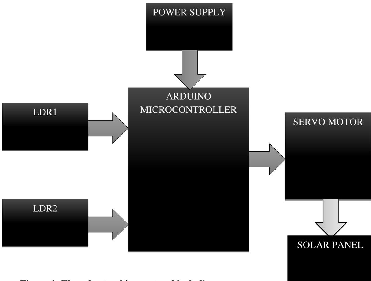
**Figure 1: The solar tracking system block diagram.**
