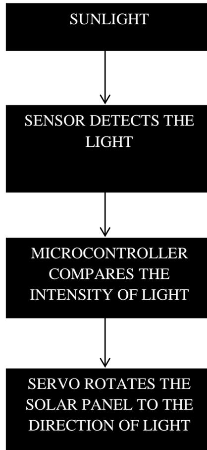
**Figure 2: Flow chart diagram of the solar tracking system**
