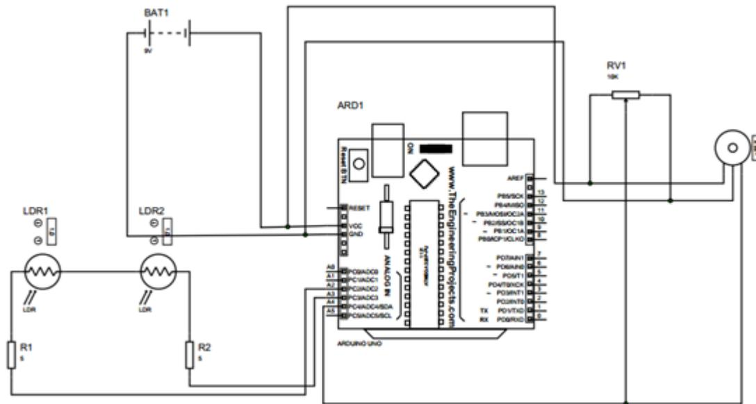
**Figure 3: Schematic diagram of the solar panel tracking system.**
