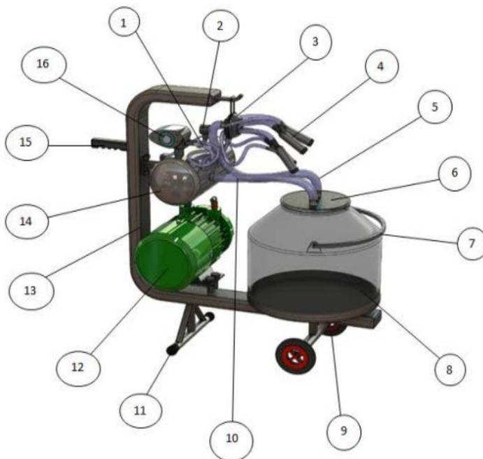
Figure 3. Parts of the machine identified.
