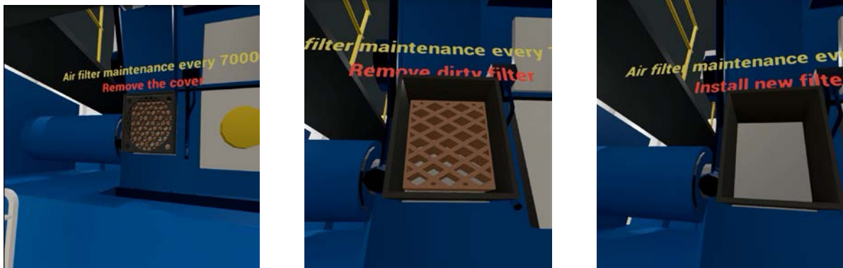
(a) Display of cover removal (b) Display of filter removal (c) Display of filter installation
