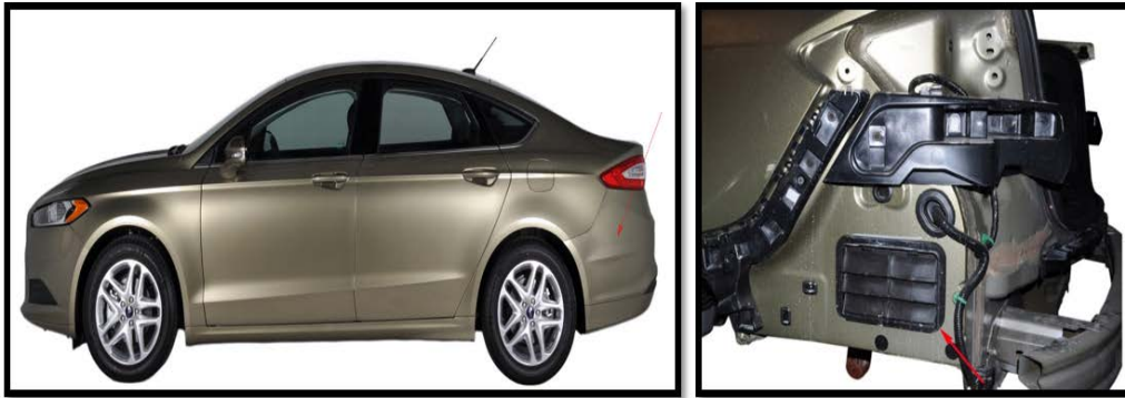
Figure 4. The Air Extractor in the Rear Quarter Panel for a Vehicle
