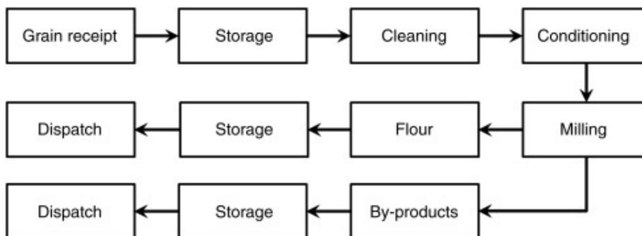
Figure 1: Flour Milling process (Alldrick, 2017)
