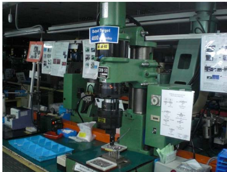
Figure 2: Radial riveting machine used to join the pin and plate lever [8]
