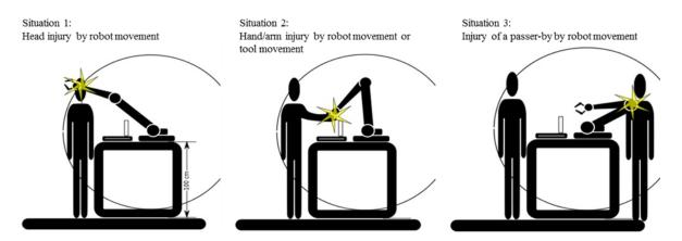
Figure 5. Identified risk situations in the hybrid assembly station
