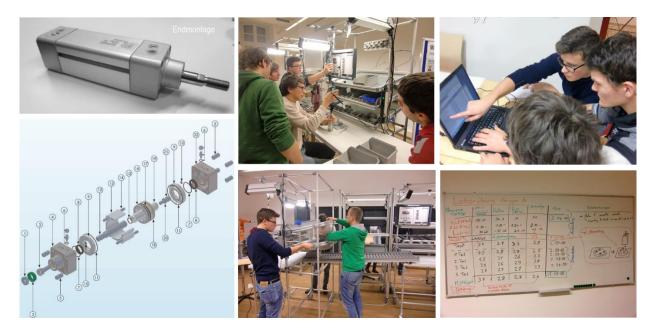
Figure 3. Case study with students: design and optimization of a manual assembly line for pneumatic cylinders
