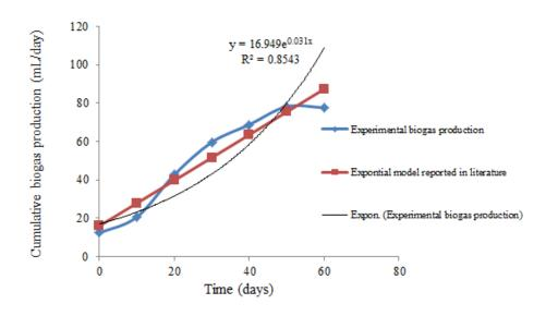
Figure 2. Comparison of the exponential kinetic model to cumulative experimental biogas data The coefficient of determination was  $R^2 = 0.83$  in the exponential model in comparison to  $R^2 = 0.93$  in the linear kinetic model. The  $R^2$  values showed that in terms of accuracy in representing the experimental data, the linear model was superior to the exponential model (Table 3).
