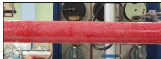
Figure 10. The sand pack saturated with red-dye-oil before flooding
