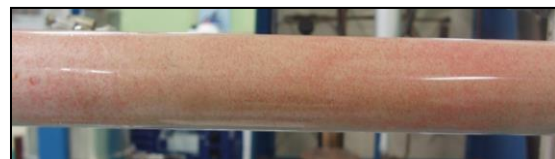
Figure 11. The sand pack after water flooding succeeded by surfactant flooding
