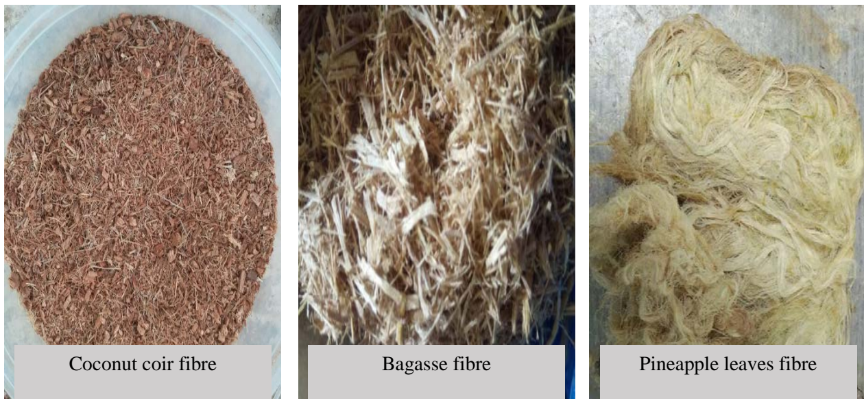
Figure 1: Extracted fibre after undergoing chemical treatment.
