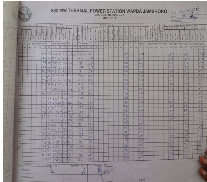
Figure 3: Chart showing values of Temperature, Pressure, Mass Flow Rate and other Variables at VARS, TPS, Jamshoro, Sindh, Pakistan
