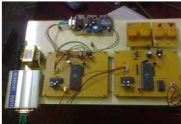
Main control unit and GSM module
