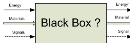
Fig 3. The conversion of energy, material and signals. Solution not yet known; task or function described on the basis of inputs and outputs, Pahl and Beitz[6]
