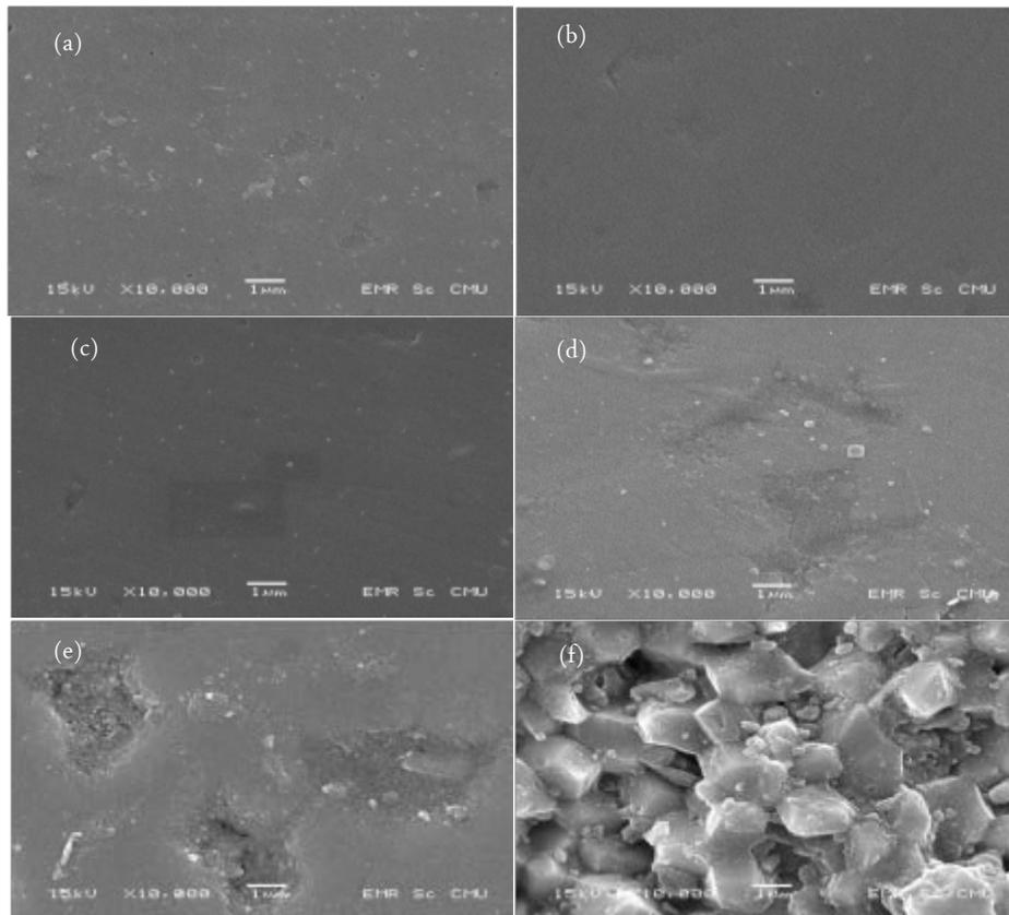
Fig. 3. . SEM of HA compact at various sintering temperature (a) 1,000 °C (b) 1,050 °C (c) 1,100 °C (d) 1,150 °C (e) 1,200 °C and (f) cross-section view of HA compact at 1,050 °C
