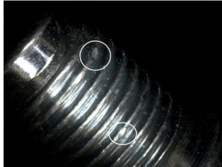
Figure 4. Small dents on bolt thread
