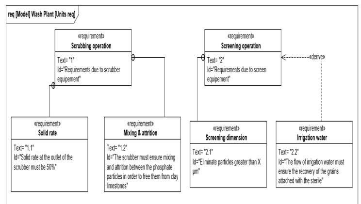
Figure 2: Different diagrams allow to capture the requirements of the Wash Plant in SysML
