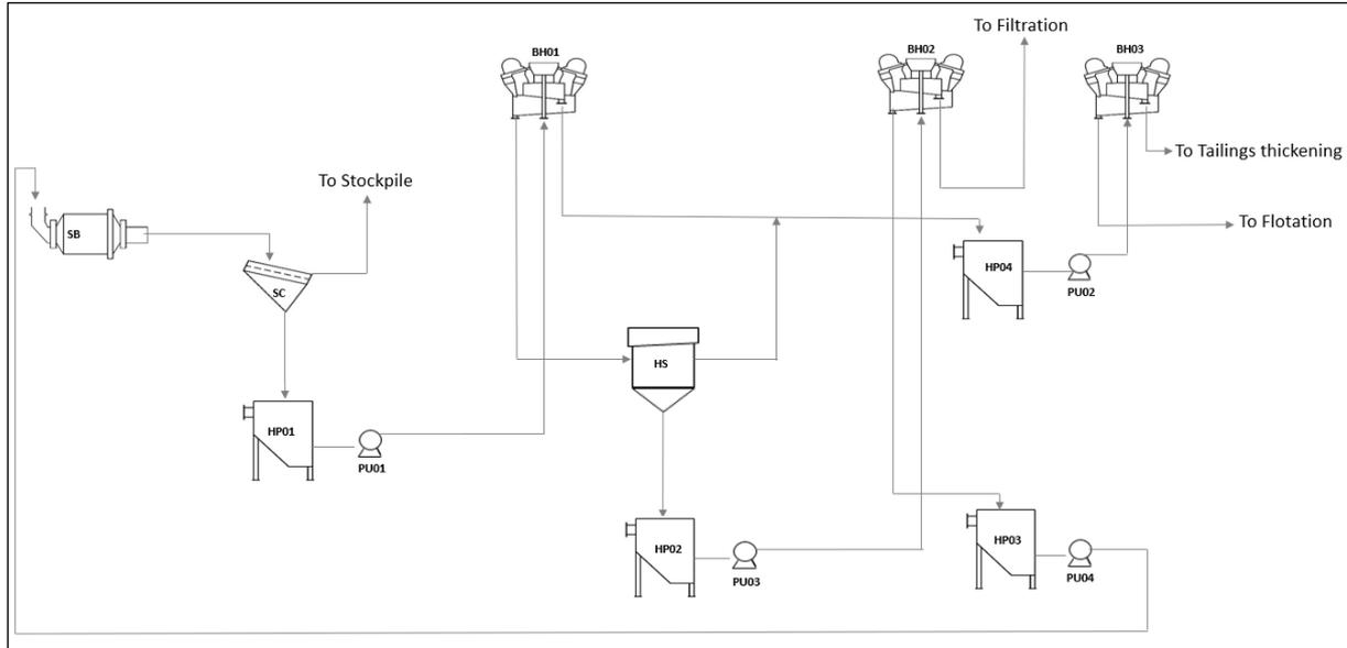
Figure 1: Simple Flowsheet of Phosphate Wash plant
