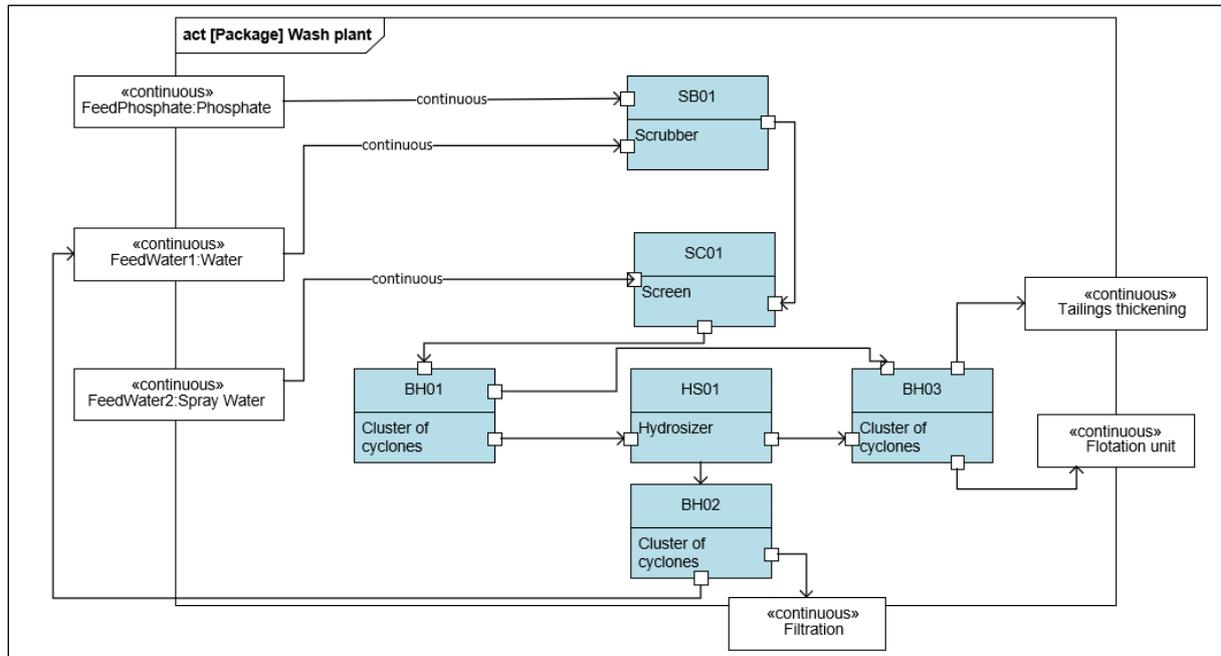
*Figure 3: Overall activity diagram of the wash Plant*
