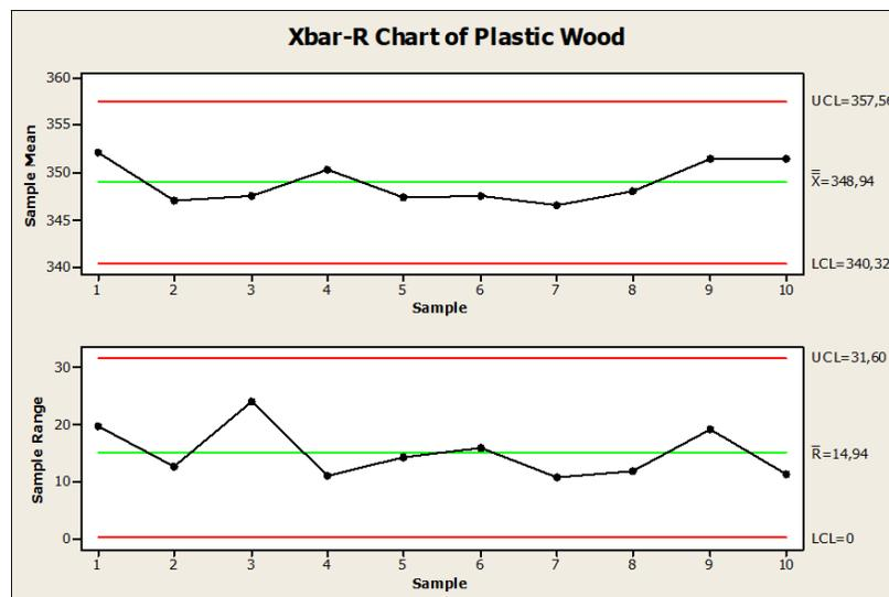
Figure 6. Graph X\_R of the production process of recycled plastic wood.
