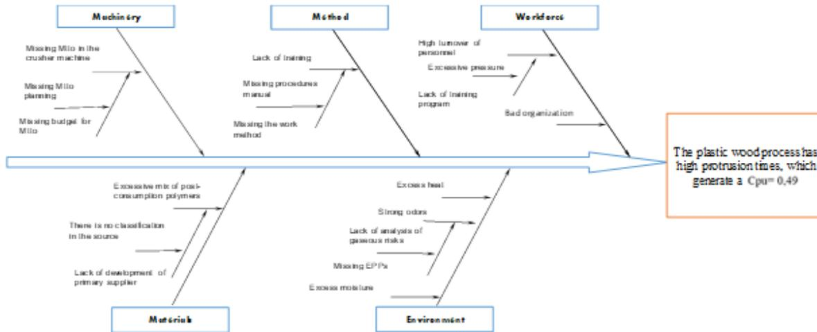
Figure 3. Cause - effect diagram of the wood plastic production process.
