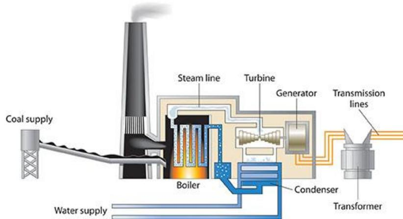
Figure 1. Main units of a coal-fired power plant
