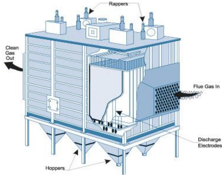
Figure 3. ESP operational process in a power plant
