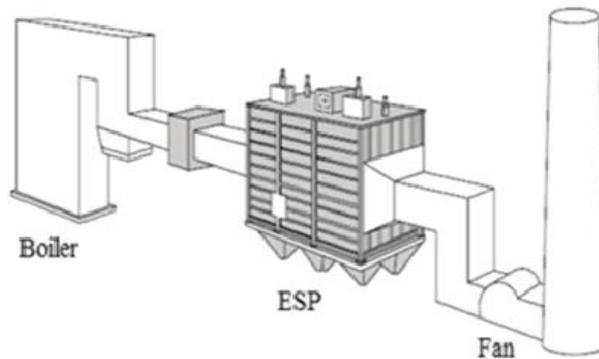
Figure 2. Placement of ESP unit in a coal-fired power plant
