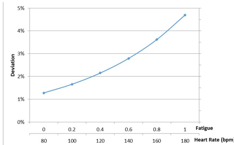
Figure 2. Graphical form of the deviation function to fatigue
