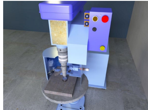
Figure 5. Final Product Design 3D Model (Higher Front view)
