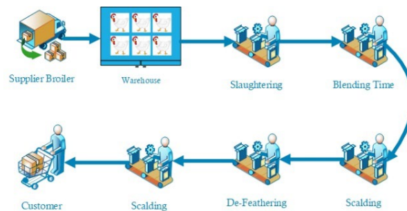
Figure 1. Production Process of Chicken Slaughterhouse
