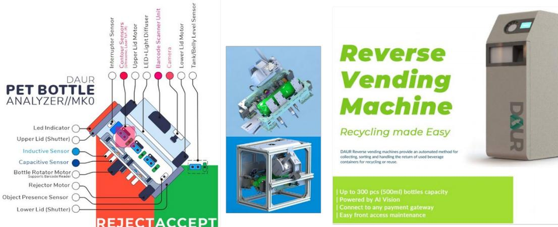
Figure 4. Prototype design of DAUR machine
