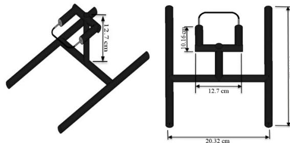
Figure 4. Isometric and Top view of the Cluster stand
