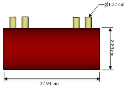
Figure 3. Side view of the vacuum accumulator
