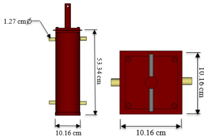
Figure 2. Front and top view of the Reciprocating Pump
