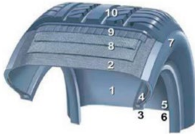
Figure 1. Cross section of a passenger car tire (Beczowska et al., 2020).
