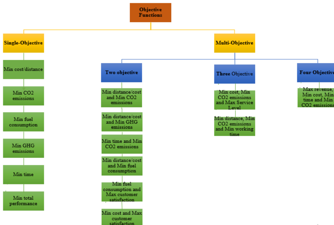
Figure 2: The framework of the objective functions in GVRP
