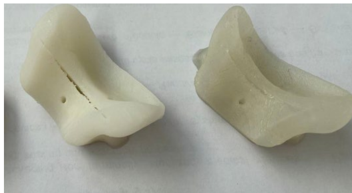
Figure 2. Cutting Guides printed by FDM in PLA (left), HTPLA (right)
