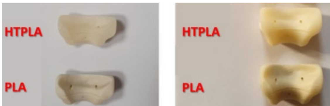
Figure 3. Comparison View of Tested Masks Before and After Sterilization Process
