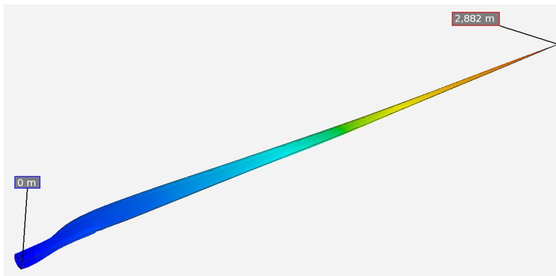
Figure 4: Expected deformation after FEA analysis.
