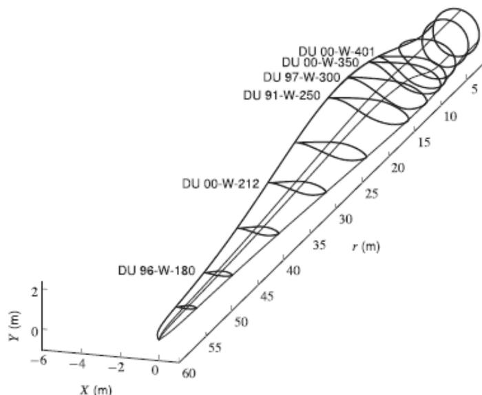
Figure 3: Wire-frame of the blade (Neto et al., 2018, p. 656, fig. 12).
