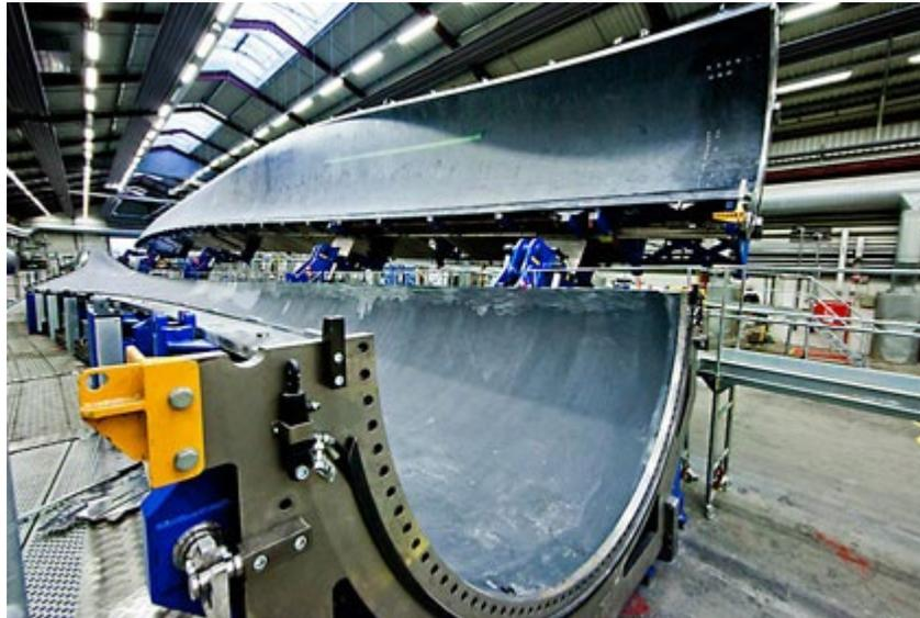
Figure 61: wind blade turbine separated in two parts, produced with classic mode.
