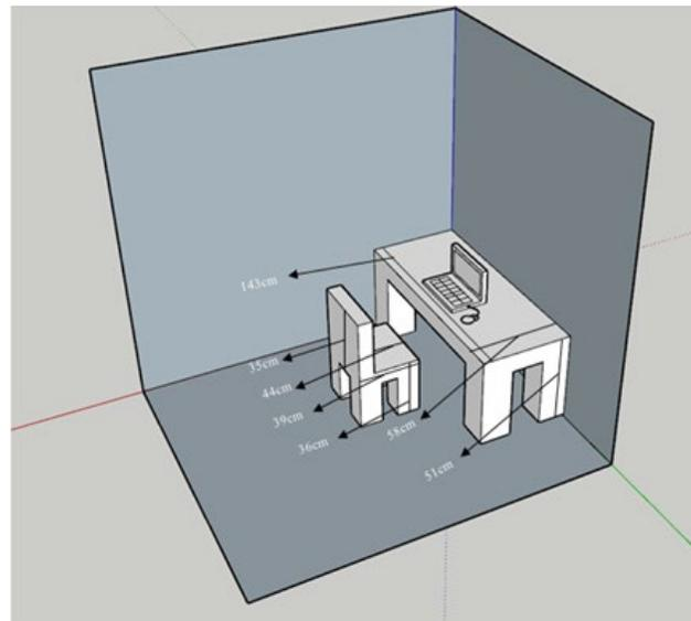
Figure 2. Recommended Design of the Computer Workstation
