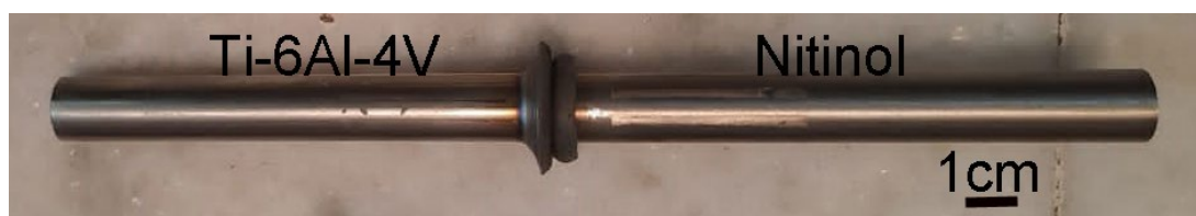
Figure 1 A successfully strong joint resulted between Ti-6Al-4V and Nitinol using the friction welding technique.
