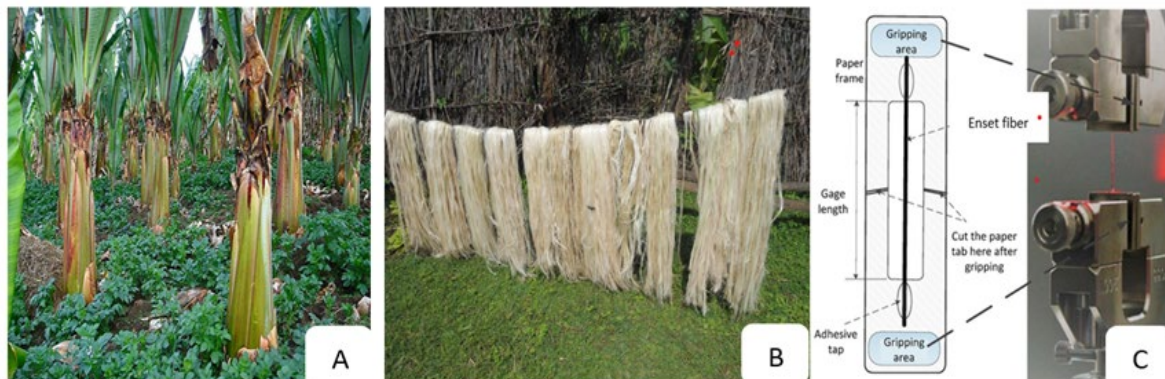
Figure 1. A-Enset Plant, B-Extracted Enset fiber, C- Fiber gripping and orientation
