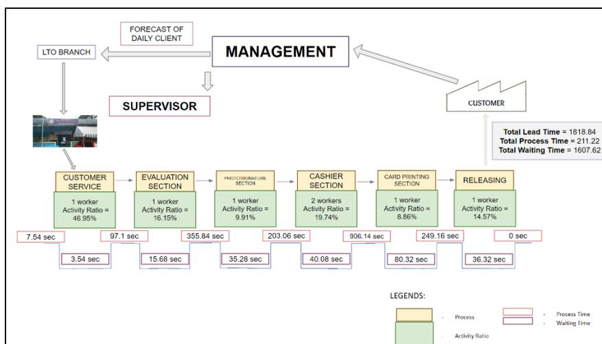
Figure 2. Value Stream Mapping of the Current System in LTO
