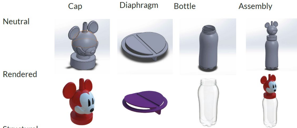
Fig 3: 3D representation and assembly images of product in neutral and rendered forms
