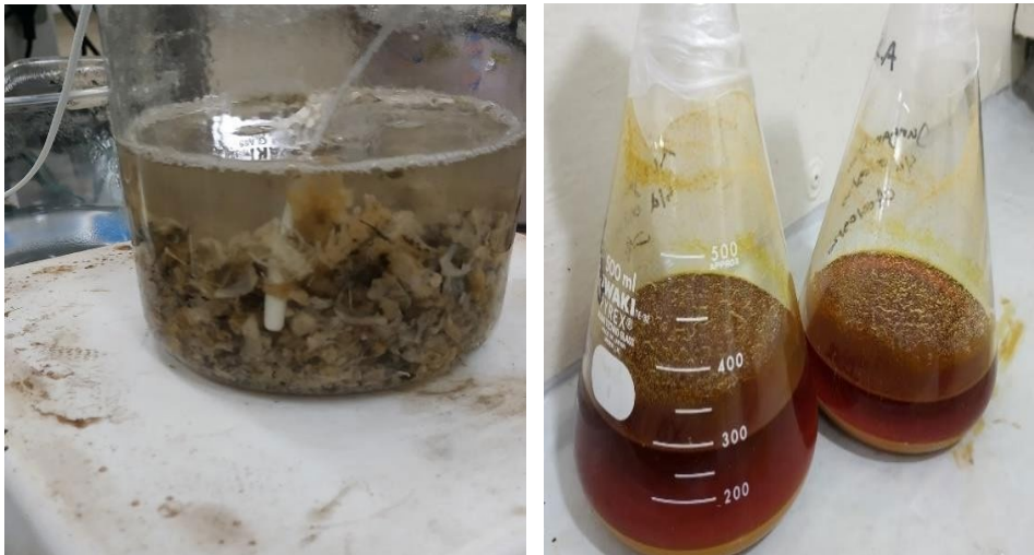
Figure 4. The images extraction of catfish bone with Aquadest 70°C for 5 hours b) The maceration extraction of turmeric with methanol 96%
