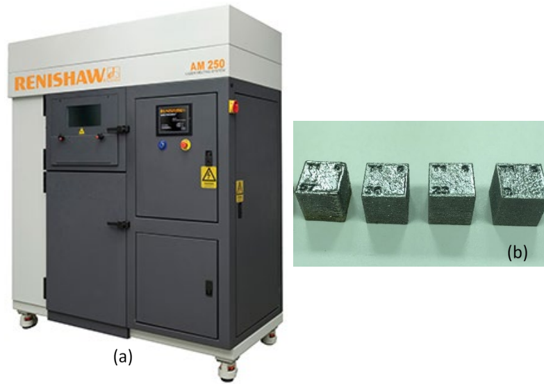
Figure 1: (a) Renishaw AM250 laser powder bed fusion machine, (b) as-build L-PBF parts
