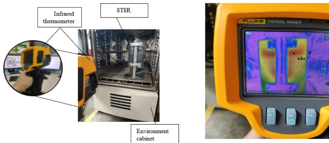
Figure 10. Thermal distribution of RRU 5G 8T8R V heatsink fin
