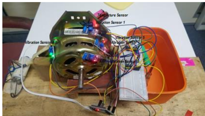
Figure 4.2b: Various Position of Sensors Attached to AC Motor
