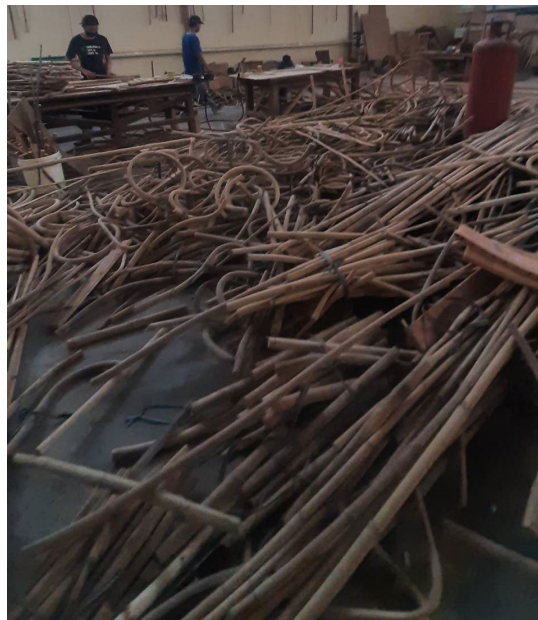
Figure 1. The Accumulation of Remaining Materials for Winston Rattan High back Armchair in the production room of PT Kharisma Rattan Mandiri
