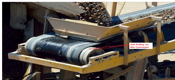
Figure 4: Typical Tail pulley Set Up (DRCrollers, n.d.).
