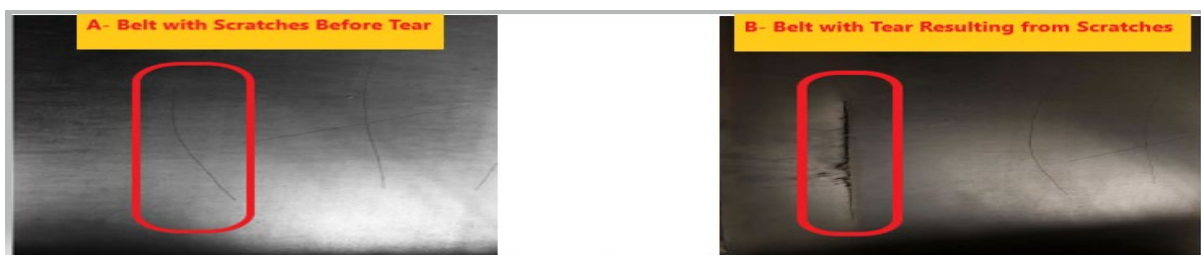
Figure 11: Belt with Scratches Before Tear (A) and Tear Resulting from Scratches (B) (Ly, et al., 2021)
