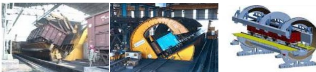
Figure 2: Typical Train Wagon Tilting Device (Anon., n.d.).
