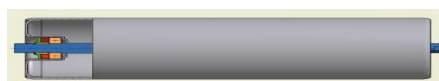
Figure 6: Idler with Bearing Assembly and a New Seal in Accordance with the Invention of the Central Mining (Sust, 2013)
