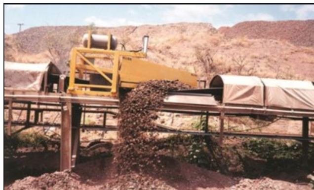
Figure 81: Straight Plough in Closed/Scraping (MARS, n.d.)
