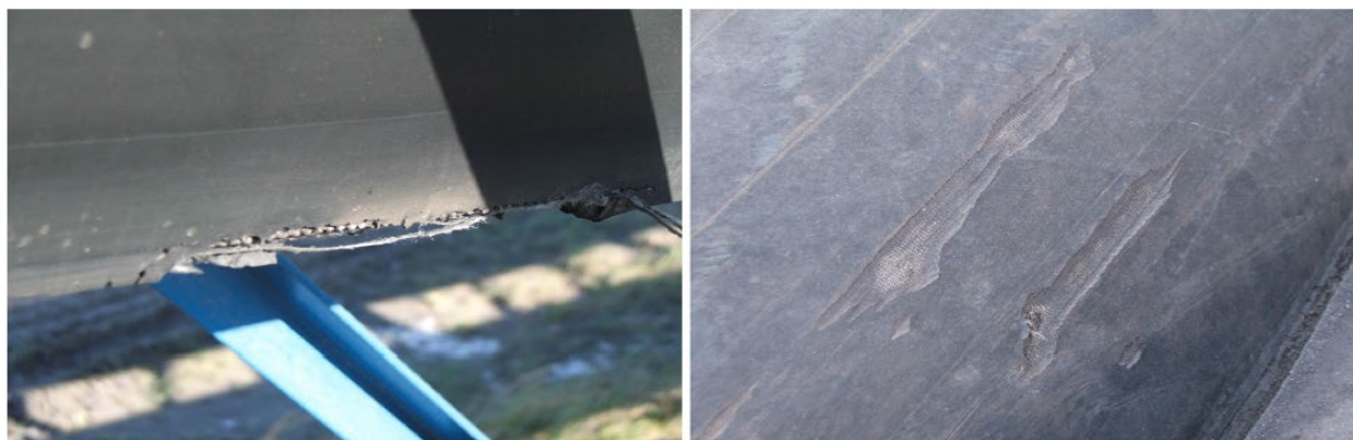
Figure 6: Example of Destructive Damage of the Rubber-Textile Conveyor Belt (Velmurugan, et al., 2021).
