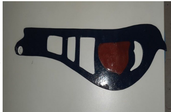
Figure 2a: Solidworks Drawing of Fuselage with Dimensions, Fig 2b: Finished Fuselage and Gear Plates
