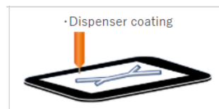
Figure 2. An example of a filling dispensing/coating method (Adapt from: https://www.dexerials.jp/en/news/2020/news20019.html )
