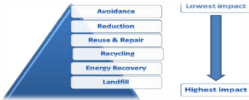
Figure 4. Hierarchy of disposal methods for e-waste (Mmereki et al 2015)
