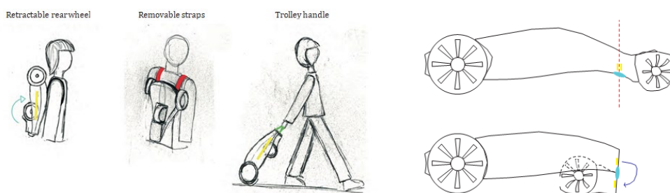
Figure 14 - Transport and closing mechanism
