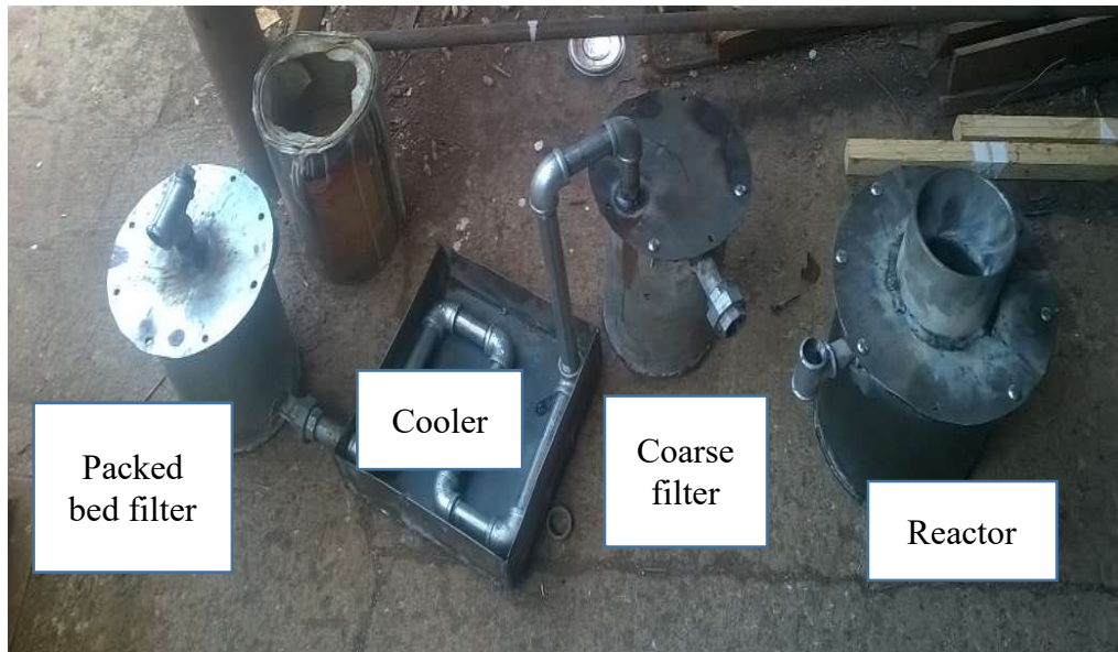
Figure 8 Fabricated Sub-Assemblies of actual prototype layout
