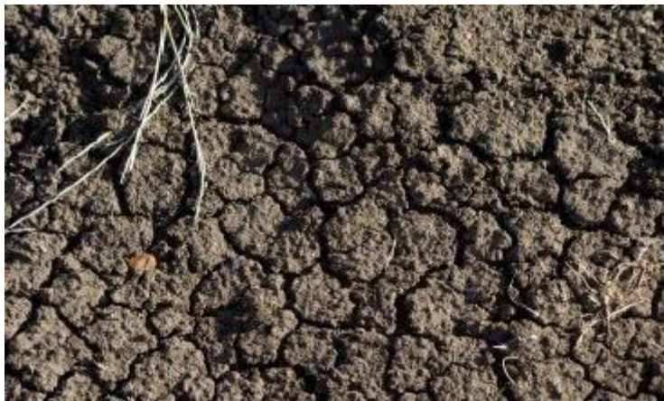
Figure 1: A picture of a black cotton soil at its drying state
